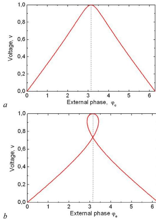
**Figure 7.** Voltage response  $v(\varphi_e)$  given by both voltage and phase dependences  $v(\psi_0)$  and  $\varphi_e(\psi_0)$  at  $i_b \equiv I_b/I_c = 2$  for  $li_{c3} \equiv 2\pi LI_{c3}/\Phi_0 = 0.58$  (a) and 1.5 (b).
