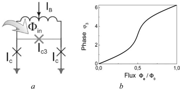
**Figure 1.** Bi-SQUID (a) and the shunt Josephson junction phase versus applied magnetic flux (b). Normalized inductance  $l = 1$ , bias current  $I_b = 2I_c$ ,  $I_{c3} = 0.85I_c$ .
