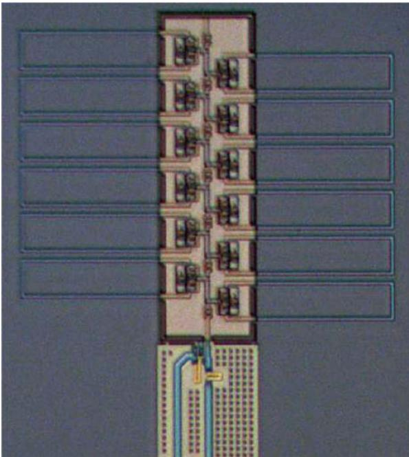
**Figure 13.** Microphotograph of the fabricated prototype of an active electrically small antenna based on a serial array of 12 bi-SQUIDs each equipped with a large superconducting loop to sense the magnetic component  $B$  of an incident electromagnetic wave. A large-size strip coil is introduced in the chip to excite a low-frequency or dc magnetic field.
