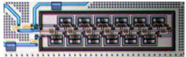
**Figure 9.** Microphotograph of serial array of 12 bi-SQUIDs.
