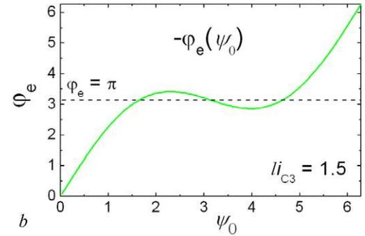
**Figure 6.** (a) Voltage dependence  $v(\psi_0)$  given by equation (6) at  $i_b \equiv I_b/I_c = 2$ ; (b) phase dependence  $-\varphi_e(\psi_0)$  given by equation (7) at  $li_{c3} \equiv 2\pi LI_{c3}/\Phi_0 = 1.5$ .
