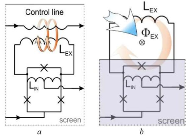
**Figure 8.** (a) Equivalent circuit of bi-SQUID with control stripline for magnetic flux application. (b) Equivalent circuit of the bi-SQUID cells implemented in a prototype of an active electrically small antenna.
