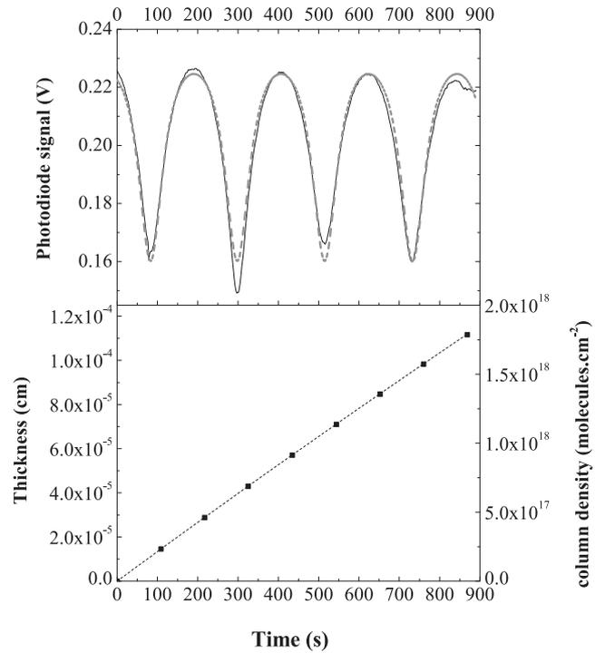
**Figure 2.** Interference pattern recorded as a function of time during the deposition of a  $\text{CH}_4$  ice film. Top panel: observed (full line) and adjusted (dashed line) interference pattern. Bottom panel: thickness and column densities (black points) calculated using a refractive index of 1.34 and a density of  $0.45 \text{ g cm}^{-3}$ .
