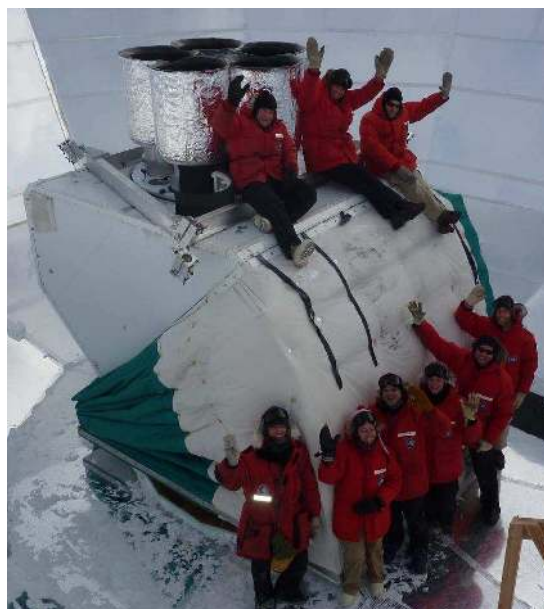
Figure 1. Keck Array telescope in February 2012, with five receivers installed in the mount originally built for DASI at the South Pole.
