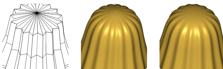
Fig. 8. Intended ripples: (left) Control net (middle) Catmull-Clark subdivision (note additional micro-ripples); (right) polar subdivision.
