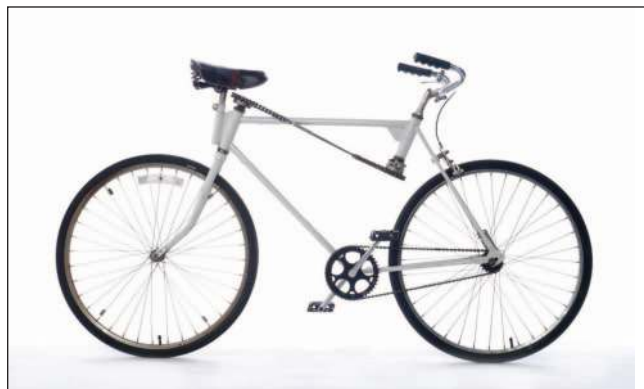
Figure 18. Klein's original unridable rear-steered bicycle. This bicycle shows the difficulties of controlling a system with poles and zeros in the right-half plane. There is a US$1,000 prize for riding this bicycle under specified conditions.
