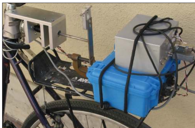
Figure 17. Rear part of the instrumented UCSB bicycle. A potentiometer is used to sense rider lean. The boxes contain a data logger and a power pack.
