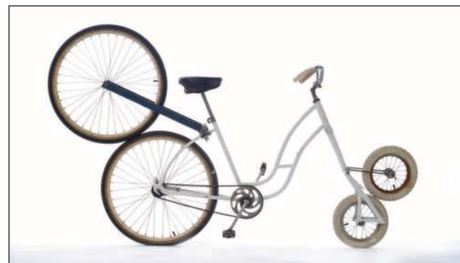
Figure 11. A UIUC bicycle with precession canceling. This bicycle is used to illustrate that gyroscopic effects have little influence on rideability.
