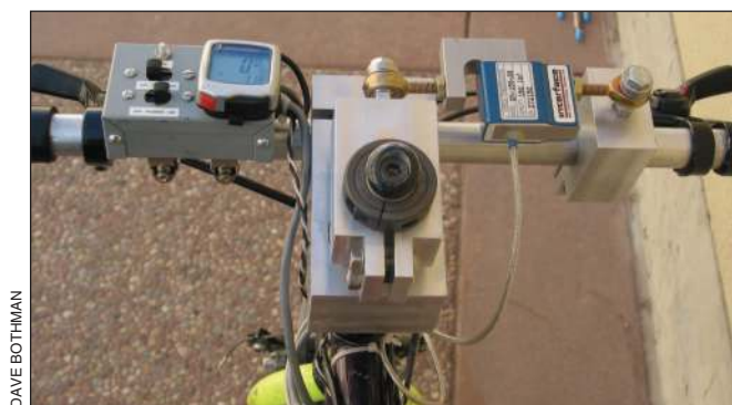
Figure 16. The handlebar of the instrumented UCSB bicycle. Steer torque is measured using a strain gauge on the right. The box on the left contains a display for speed and switches for data logging.
