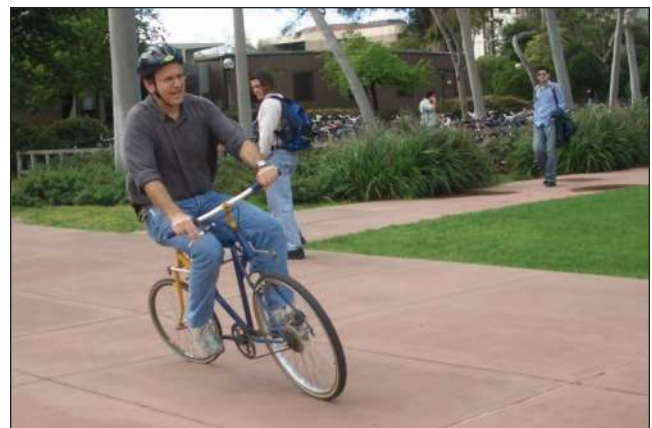
Figure 20. The UCSB rear-steered bicycle. This bicycle is rideable as demonstrated by Dave Bothman, who supervised the construction of the bicycle. Riding this bicycle requires skill and dare because the rider has to reach high speed quickly.
