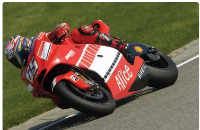
FIGURE 7 Loris Capirossi riding the Ducati Desmosedici GP5. Ducati Corse's MotoGP racing motorcycle is powered by a V-4 four-stroke 989-cc engine. The vehicle has a maximum output power of approximately 161 kW at 16,000 rpm. The corresponding top speed is in excess of 90 m/s. (Reproduced with permission of Ducati Corse, Bologna, Italy.)
