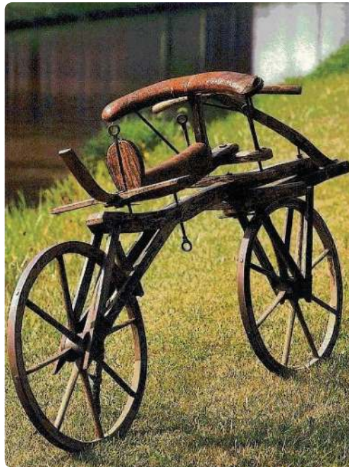
FIGURE 1 The draisine, or running, machine. This vehicle, which was first built in Germany in 1816, is early in a long line of inventions leading to the contemporary bicycle. (Reproduced with permission of the Bicycle Museum of America, New Bremen, Ohio.)
