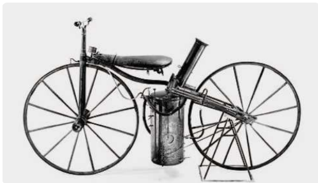
FIGURE 4 Sylvester Roper steam motorcycle. This vehicle is powered by a two-cylinder steam engine that uses connecting rods fixed directly to the rear wheel. (Reproduced with permission of the Smithsonian Museum, Washington, D.C.)
