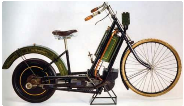
FIGURE 6 Hildebrand and Wolfmüller motorcycle. This machine, patented in 1894, was the first successful production motorcycle. (Reproduced with permission of the Deutsches Zweirad- und NSU-Museum, Neckarsulm, Germany.)
