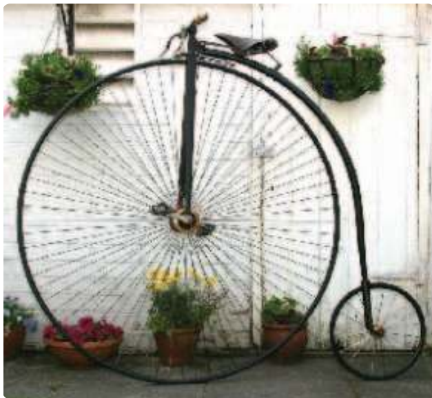
FIGURE 3 Penny farthing, or ordinary. This bicycle is believed to have been manufactured by Thos Humber of Beeston, Nottinghamshire, England, circa 1882. The braking limitations of this vehicle's layout are obvious! (Reproduced with permission of the Glynn Stockdale Collection, Knutsford, England.)
