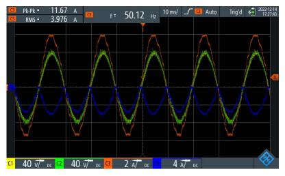
**Figure 7.** System parameters during grid-parallel operation with a  $V_{\text{grid}}$  of 56 V RMS,  $I_{\text{sys}}$  of 4 A RMS and a grid frequency  $f_{\text{grid}}$  of 50 Hz. Grid voltage (green), inverter voltage (yellow), inverter current (red) and current of a single battery cell (blue).
