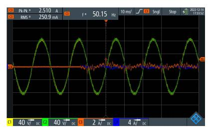
**Figure 8.** System parameters at operation startup with a  $V_{\text{grid}}$  of 56 V RMS,  $I_{\text{sys}}$  of 0 A RMS and  $f_{\text{grid}}$  of 50 Hz. Grid voltage (green), inverter voltage (yellow), inverter current (red) and current of a single battery cell (blue).
