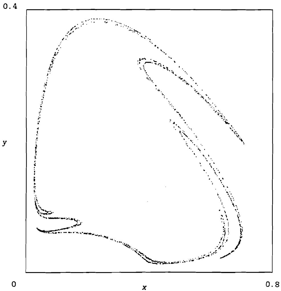
Fig.3. A strange attractor of system (5)-(7) appearing through torus destruction. The parameter values are r = 0.73 \cdot 2\pi , b_0 = 0.28 , e = 1 , a = 2 \cdot 2\pi , d = 2\pi , \varepsilon = 0.35 .
