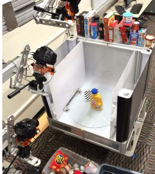
Fig. 1. Our data-collection system. We place the object near the center of the turntable, and our software takes care of the rest. Note the chessboard on the turntable to merge clouds as the turntable moves. Sample objects from the dataset can be seen sitting on top of the Ortery Photobench.
