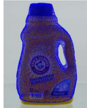
Fig. 8. The 3D mesh is projected onto one of the Canon images.
