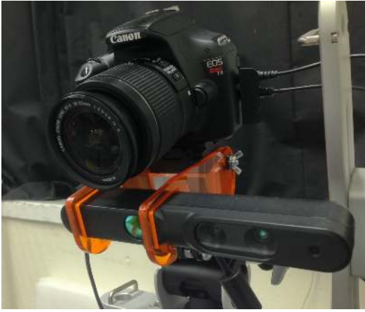
Fig. 2. Carmine mounted to Canon T3 using RGBDToolkit mount.
