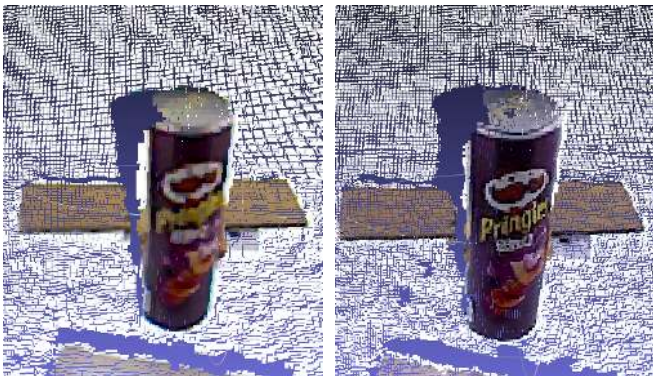
Fig. 4. Comparison of hardware and software registration. The left image shows a hardware-registered point cloud. Note the bleeding of the cardboard in the background onto the Pringles can and the low resolution of the color data. The right image shows a software-registered point cloud using our calibration. Most of the bleeding of the cardboard onto the can has been fixed, and we can use higher-resolution color data.
