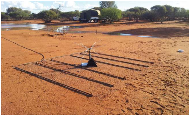
Figure 4. The BIGHORNS antenna and the front-end box (in the foreground) separated by 100 m of RF-cable from the camper trailer housing an RF-shielded rack with the back-end electronics (in the background) as deployed at the Wondinong Station in April 2014.
