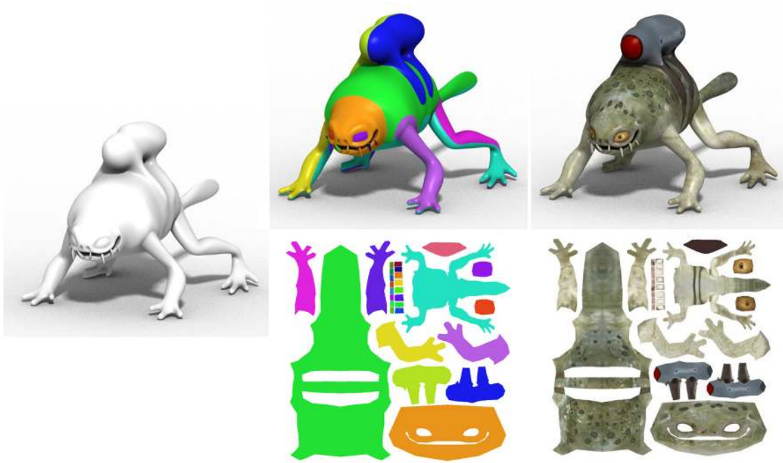
Figure 1.1: 3D surface of a monster frog rendered using just lighting and geometry(left). The surface split into several charts (top middle) and its corresponding parameterization into 2D texture space (bottom middle). The surface rendered with texture mapping (top right), and the corresponding texture image (bottom right).
