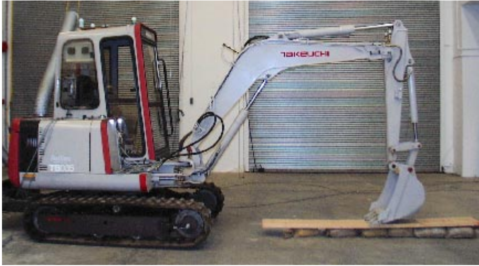
Figure 4: Photograph of the UBC mini-excavator performing a leveling task on a piece of lumber.
