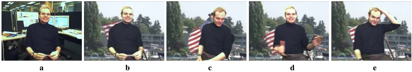
Figure 8. Bilayer segmentation and background substitution. (a) A frame from the MS test sequence; (b,...,e) foreground extraction and anti-aliased background substitution, over several frames. (e) The algorithm is capable of handling complex motions.
