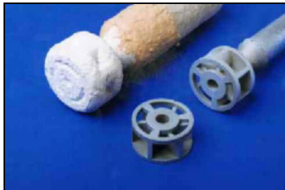
Figure 5 SLS-produced investment casting shell for impeller wheel (source: Fraunhofer Institute IPT)
