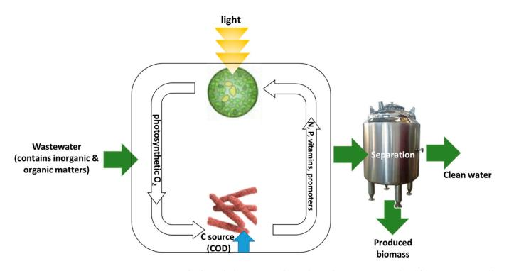
**Figure 2.** Main biological phenomena taking place when using microalgae/bacteria consortia for nutrients' recovery from wastewater effluents (redrawn from [22]).
