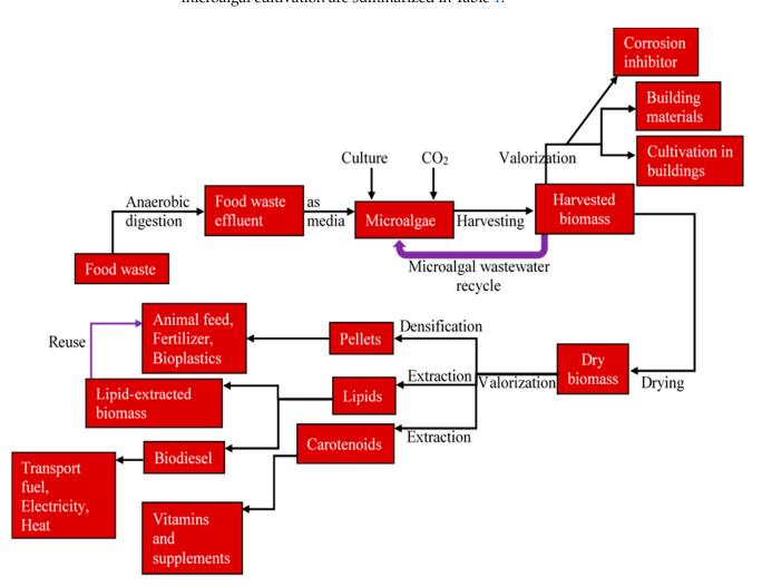
Figure 3. Simplified pathways of utilizing microalgae cultivated from food waste effluents.
