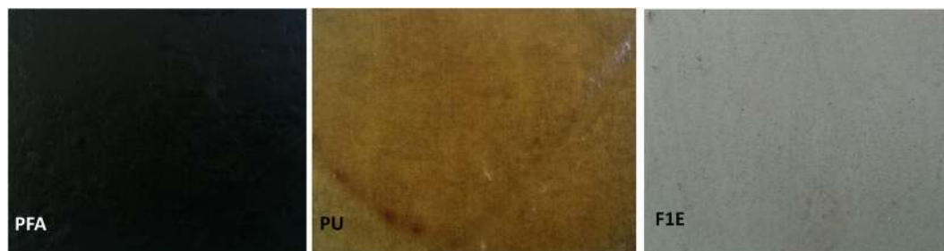
Figure 1. Flax/Phenolic laminates coated with polyfurfuryl alcohol (PFA), polyurethane (PU) and FIRESHELL® (F1E).
