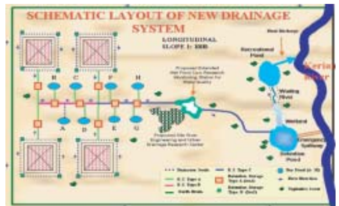
Figure 11 Schematic layout of BIOECODS.
