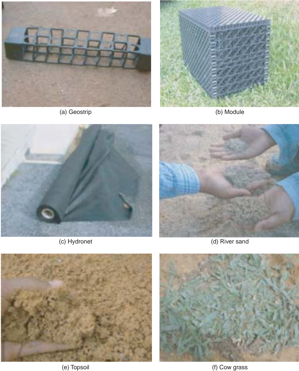
Figure 32 Materials used for the construction of ecological swales.
