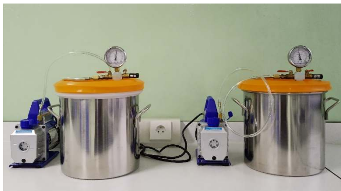
Fig. 2. A set of vacuum chamber for impregnation of ramie fibers with Bio-PU resins.
