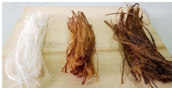
Fig. 9. Photograph of ramie fibers before impregnation (left), after impregnated with Bio-PUL-EtAc (center), and after impregnated with Bio-PU-L-MeOH (right).
