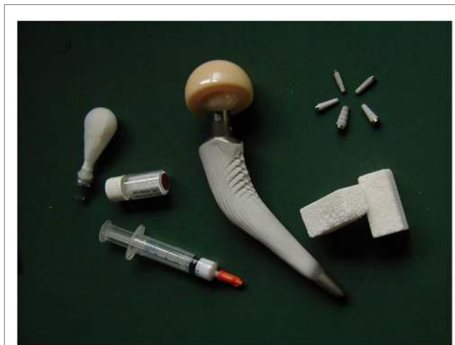
FIGURE 1 | Examples of commercial bioceramics for medical applications: powders and granules for use as bone fillers (typically calcium phosphates or bioactive glass), hemispherical acetabular cup (alumina) for hip joint prosthesis, hydroxyapatite coating on femoral metal stem, porous scaffolds (usually calcium phosphates or bioactive glass/glass-ceramic). Image reproduced from © Dorozhkin (2010a).
