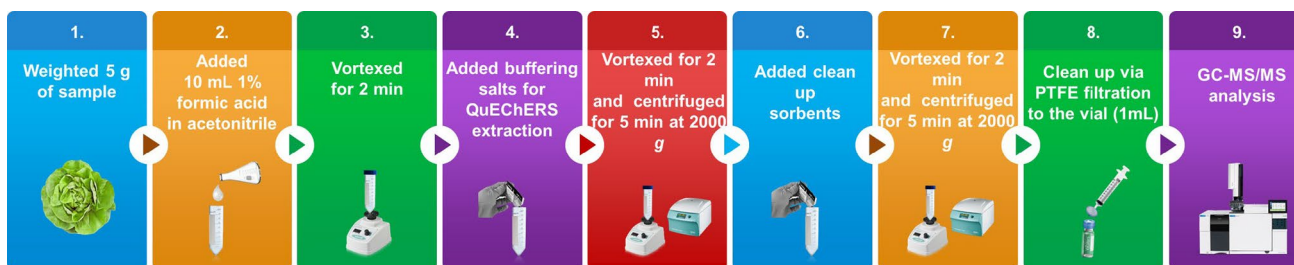
Fig. 1 Detailed extraction and determination procedure of fungicides from lettuce
