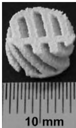
Figure 3. Printed test structure HA-S after sintering.
