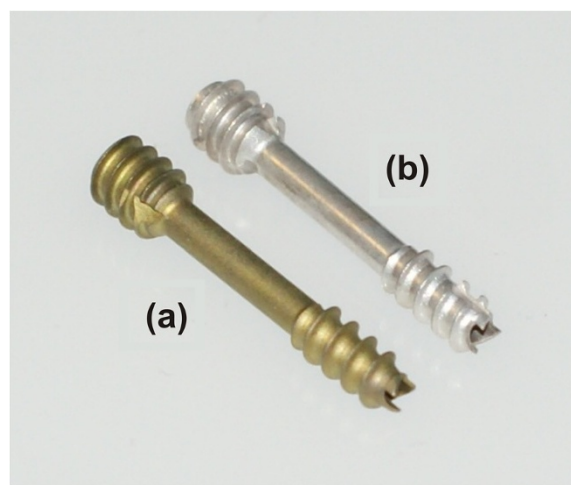
Figure 1 The two cannulated screws with the same design. a) The titanium screw (Fracture compressing screw, Königsee Implantate GmbH, Am Sand 4, 07426 Allendorf, Germany), b) MAGNEZIX® Compression Screw (Syntellix AG Schiffgraben 11, 30159 Hannover, Germany).
