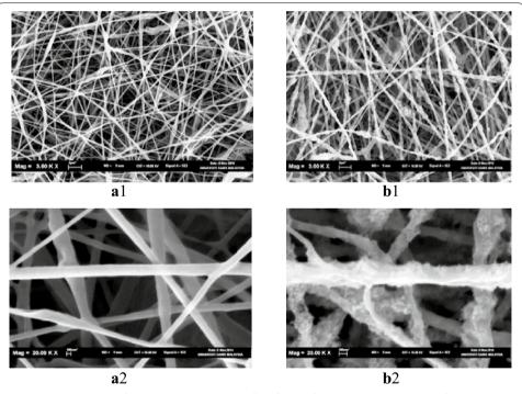
**Fig. 5** SEM micrographs for PHB and PHB–TiO<sub>2</sub> nanofiber films before degradation. **a1** PHB before degradation, **b1** PHB–TiO<sub>2</sub> nanofiber before degradation, **a2** PHB before degradation, **b2** PHB–TiO<sub>2</sub> nanofiber before degradation
