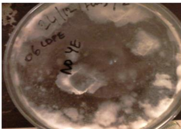
Figure 2. LDPE film showing colonization of hyphae.
