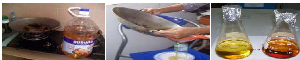
Fig. 5.2. Waste cooking palm oil, waste palm oil collection, palm biodiesel (Upper layer) and lower layer is glycerin
