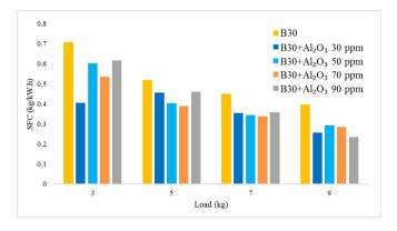
Figure 7. Specific fuel consumption at different engine loads
