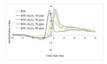
Figure 8. Net heat release at crank angle
