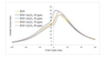
Figure 9. Cylinder pressure at crank angle
