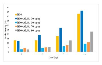
Figure 11. Smoke opaciity at different engine loads
