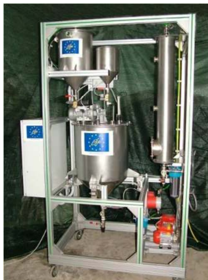
Figure-3 Pilot plant for biodiesel production [8]
