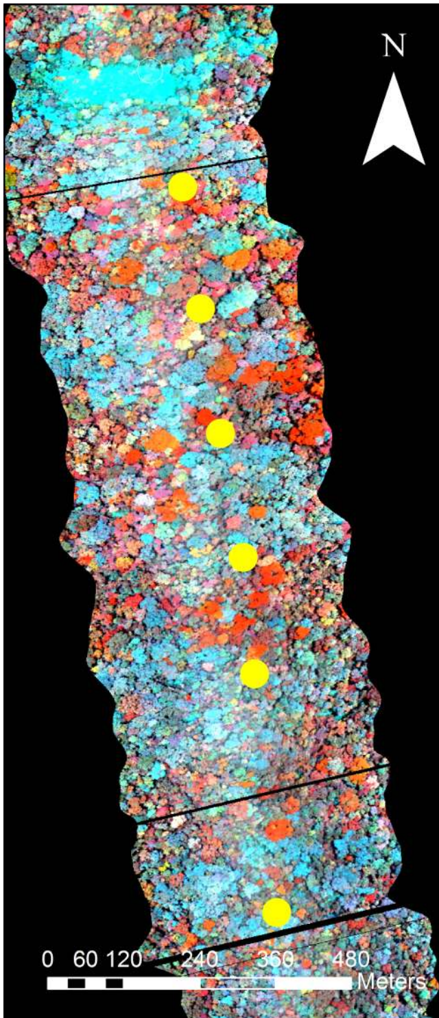
Figure 2. A strip of hyperspectral data (in false-color composite at 807.5 (R), 597.3 (G) and 467.3 (B) nm) showed as an example of available imagery, and with overlapped field plots areas, colored in yellow.
