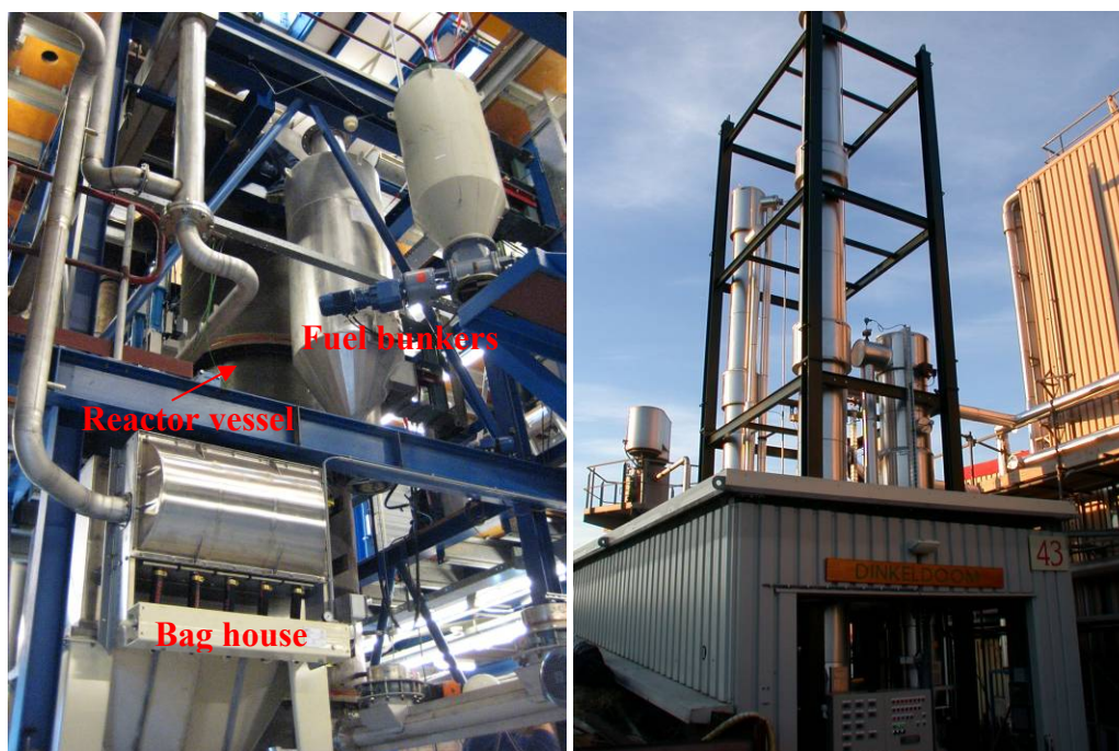
Figure 5. Photos of pilot scale MILENA (left) and OLGA (right)
