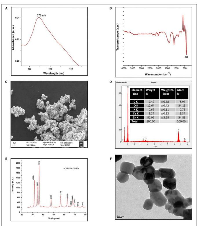
FIGURE 2 | Characterization of SaZnO-NPs. (A) UV-Visible spectrum of SaZnO NPs, (B) FTIR spectrum of SaZnO NPs, (C) SEM micrograph of SaZnO NPs, (D) EDX pattern of SaZnO NPs (E) XRD pattern of SaZnO NPs, (F) TEM micrograph of SaZnO NPs.
