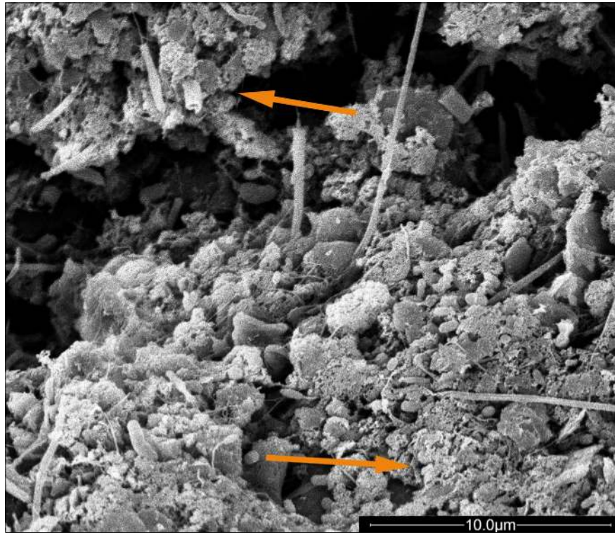
Figure 9. SEM micrographs of biofilms in emitter flow path after 144 h of irrigation with reclaimed wastewater (5000×).
