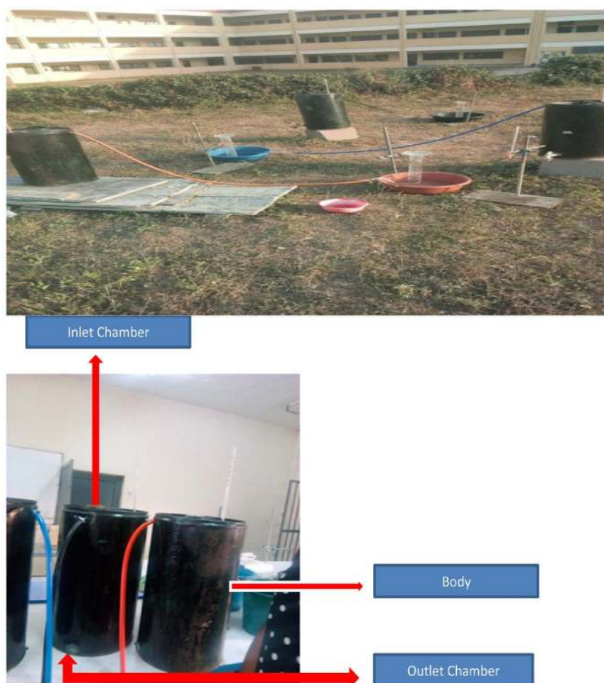
Figure 1. Experimental set up with 30 L bio-digester.
