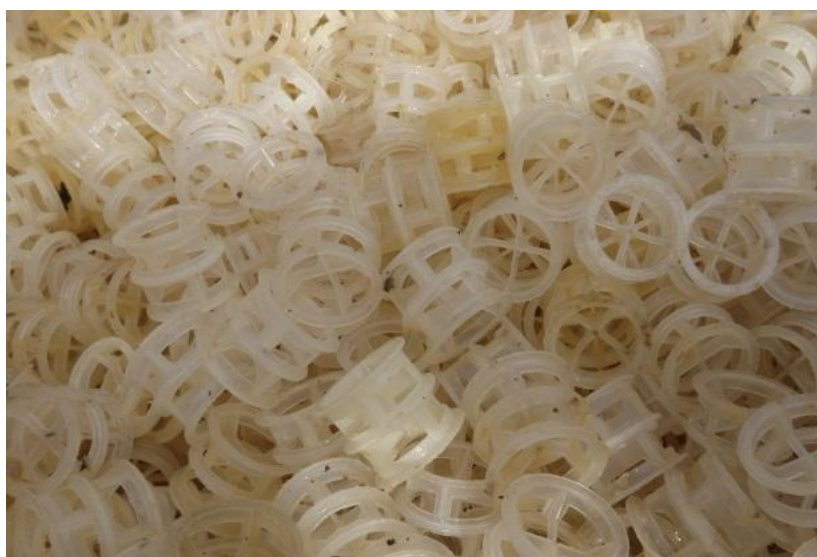
Figure 21 A typical design of random packing which is used in water scrubber absorption columns. Image from Malmberg Water.
