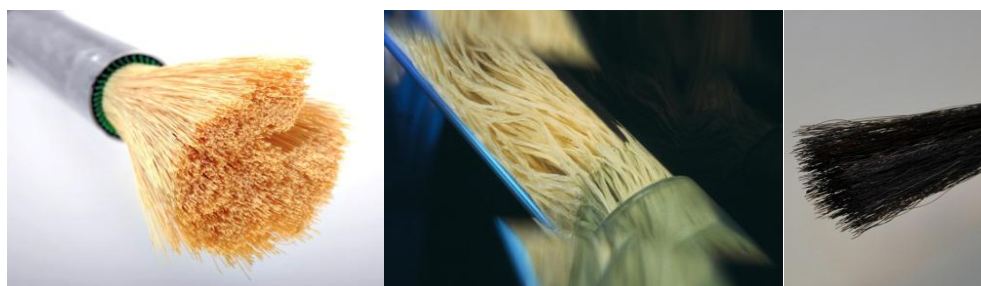
Figure 13 Hollow fibre membrane from Evonik Sepuran to the left, from Air Liquide Medal in the middle and carbon membrane from Memfoact to the right. Images from Evonik Fibres, Air Liquide and Memfoact.
