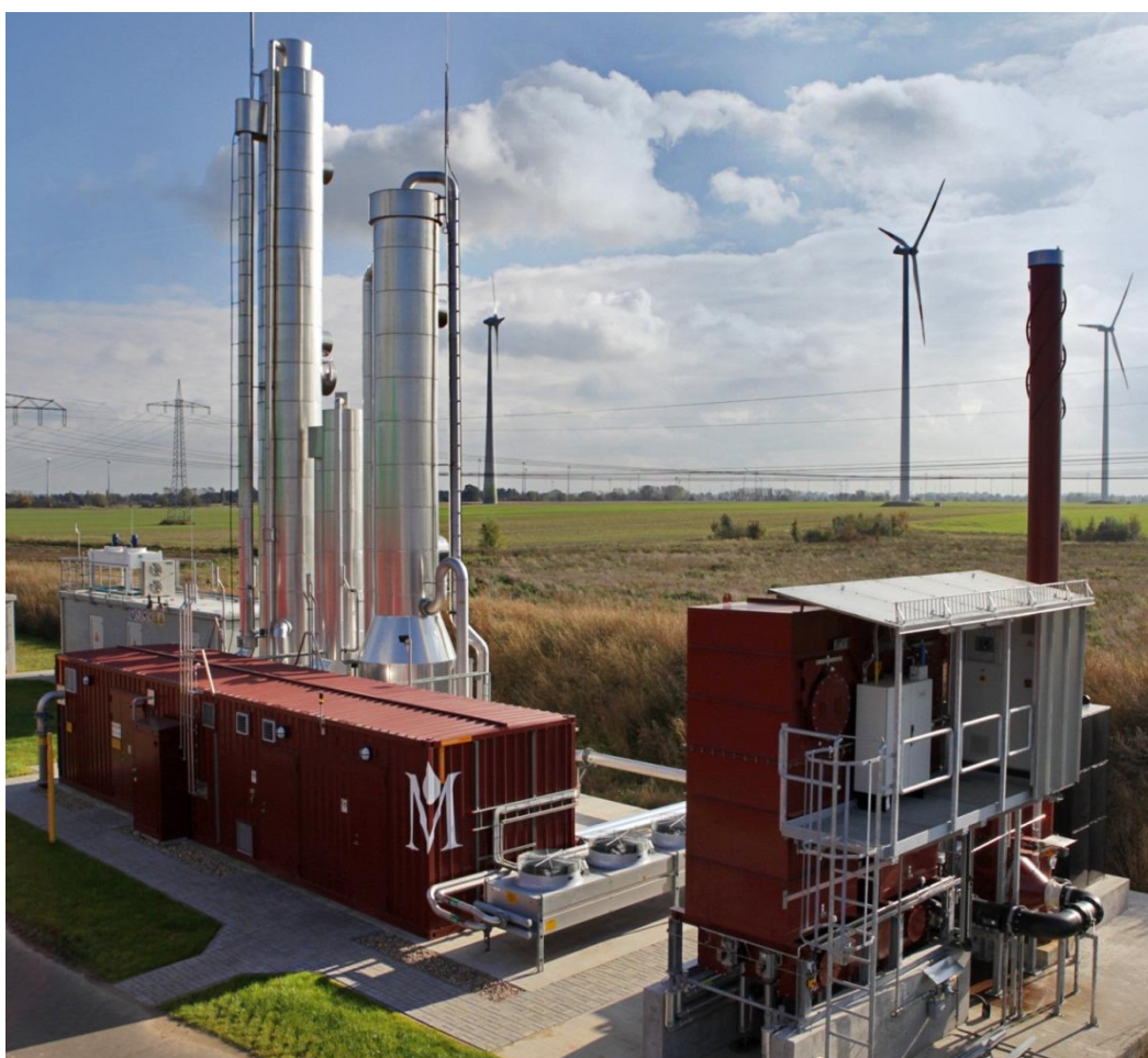
Figure 20 A water scrubber for biogas upgrading. The two towers are the absorption and desorption columns. The scrubber is equipped with an RTO unit which is shown to the right in the photograph. Image from Malmberg Water
