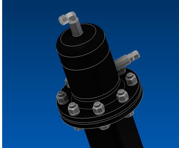
Figure 6-4 - Endcap of test column with fittings
