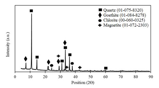
**Figure 1.** XRD pattern of oxide gold ore.
