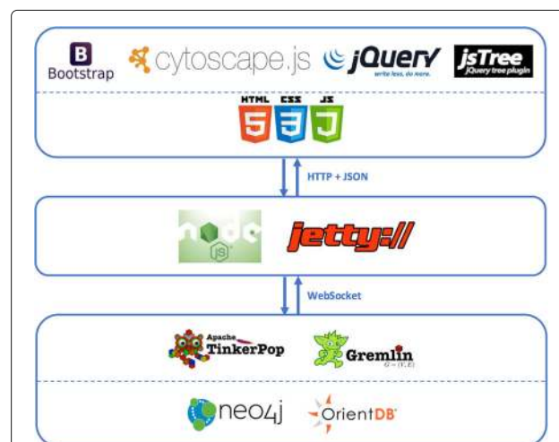
Fig. 2 BioGraph architectural stack. The picture gives an overview on the state-of-the-art technology behind BioGraph. Used tools are grouped into three levels. From the bottom to the top: the Graph Data level overlooked by Apache Tinkerpop, the Microservices level, and the Web Application level. Protocols and data formats of inter-level communications are also highlighted
