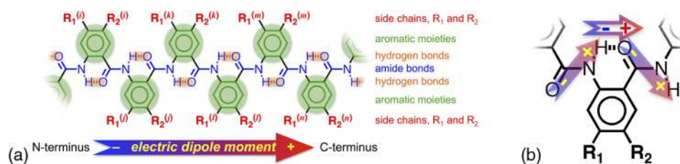
Fig. 1 Bioinspired molecular electrets composed of anthranilamide (Aa) residues: (a) a segment of a molecular electret—Aa (i) —Aa (j) —Aa (k) —Aa (l) —Aa (m) —Aa (n) ; (b) origin of the Aa dipole from ordered orientation of amide bonds and from the polarization upon hydrogen bonding.
