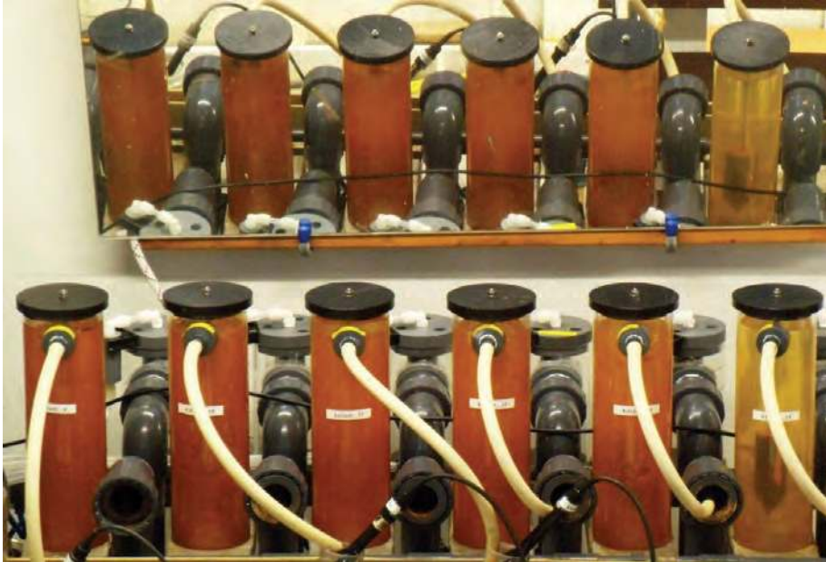
Figure B.1: Picture of the oxidation columns' setup after seven weeks; left to right: pH of the influent 6.5 to 8.25
