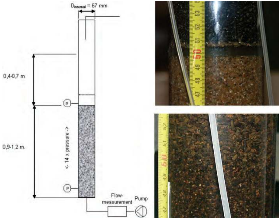
Figure 3: Diagram (left) and photos (fresh materials top right and coated materials bottom right) of experimental setup for media expansion measurements
