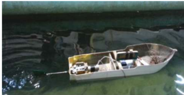
Figure 24. Remotely operated surface ship model in the self-propelling mode.
