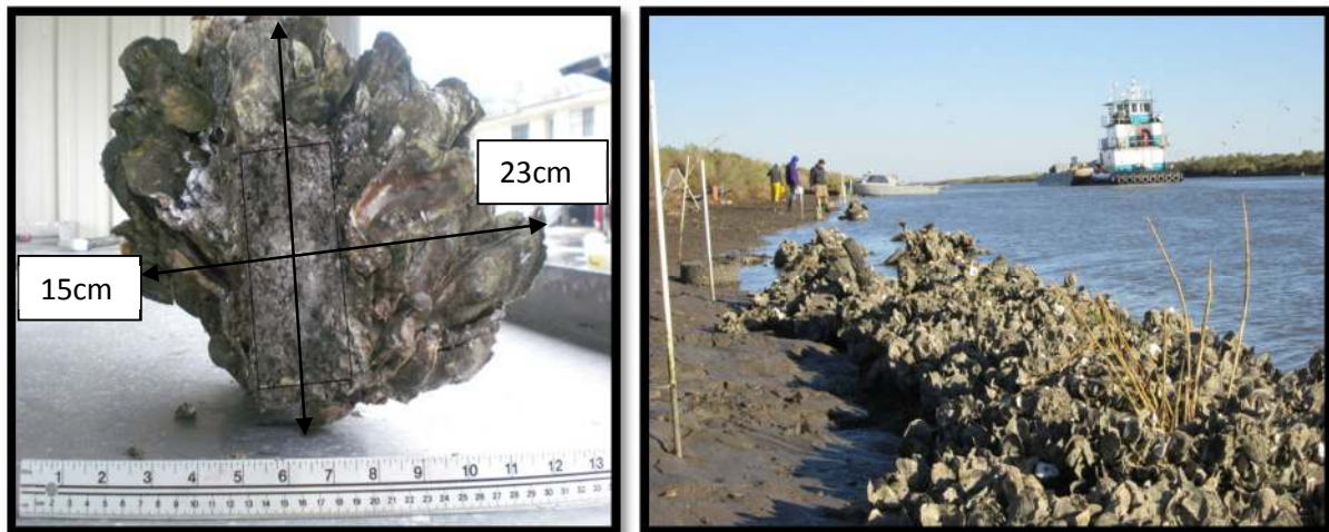
Figure 2.2 a, b: (a) Cross section of concrete oyster reef ring (2009), from (b) existing biologically dominated ring reef.
