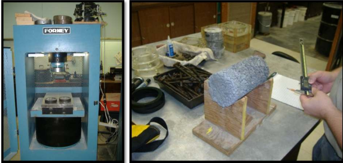
Figure 3.9 a, b: (a) FX Series Forney Premium Compression Machine, and (b) batch test cylinders.
