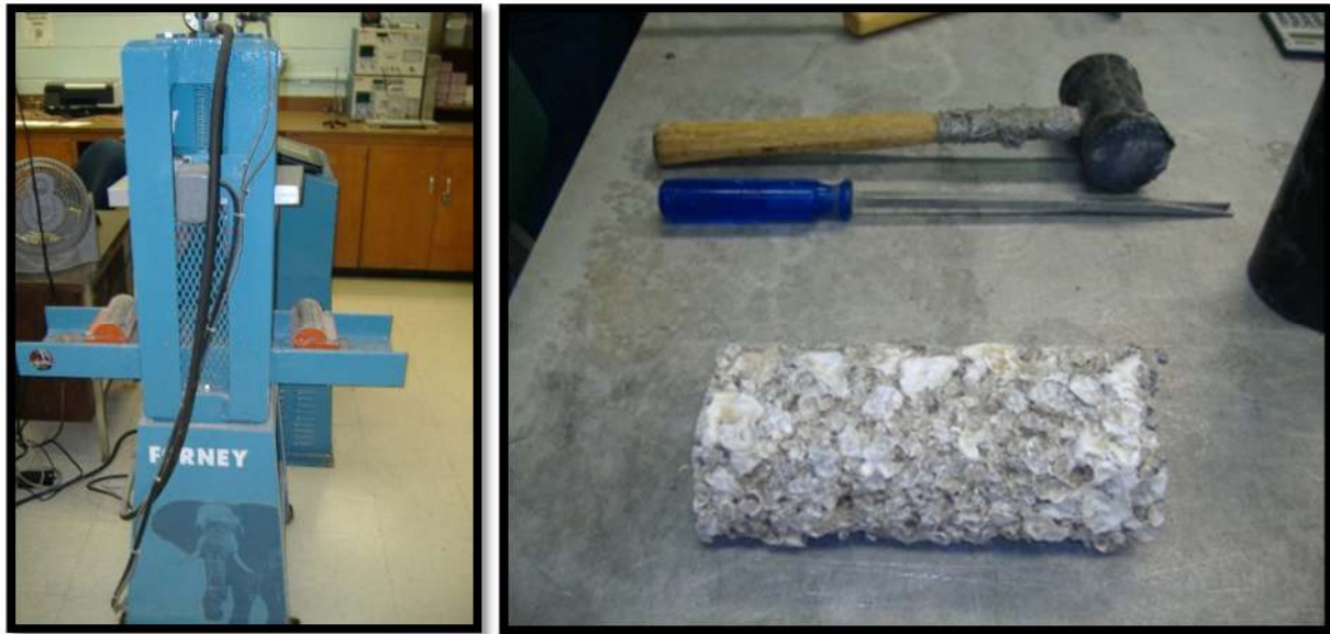
Figure 3.11 a, b: (a) Standalone Forney Beam Tester and (b) log specimen.
