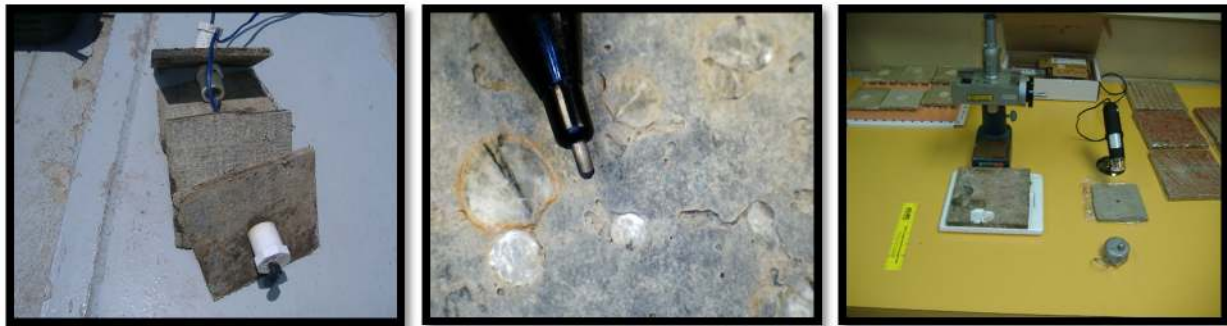
Figure 2.4 a, b, c: (a) Spat plate configuration (b) Veho™ digital microscope imagery, and (c) dissecting microscope lab set-up (Risinger, 2011).
