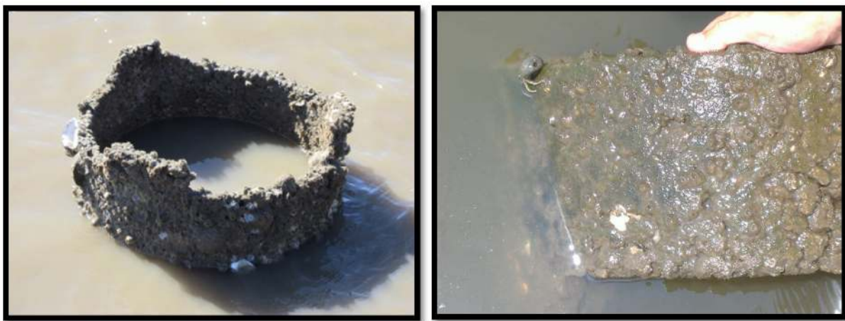
Figure 2.10 a, b: (a) Biofouling on ring in lower intertidal zone (b) Biofouling on ring in upper intertidal zone emplaced during summer months (Risinger, 2011).
