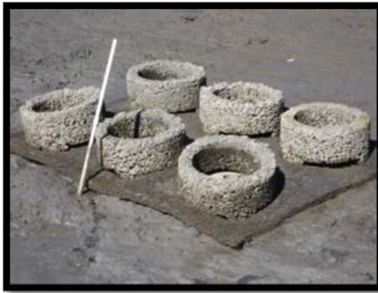
Figure 4.8 a, b: (a) Six-ring emplacement with geotextile fabric liner and (b) Tabular sediment survey data (in meters) AMSL at Site 4-M
