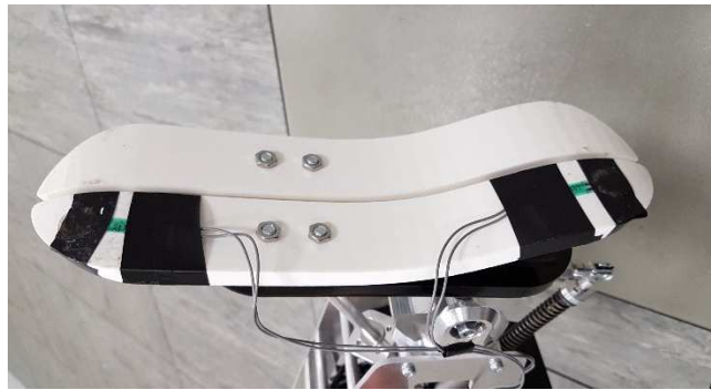
Fig. 9. Heel and toe pressure sensors.
