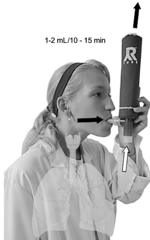
Figure 1. Exhaled breath condensate schematic. As the individual inhales, air flows into the device, bypassing the cooling sleeve, as indicated by the white arrow. During exhalation air moves out through the cooling chamber as indicated by the black arrows.
