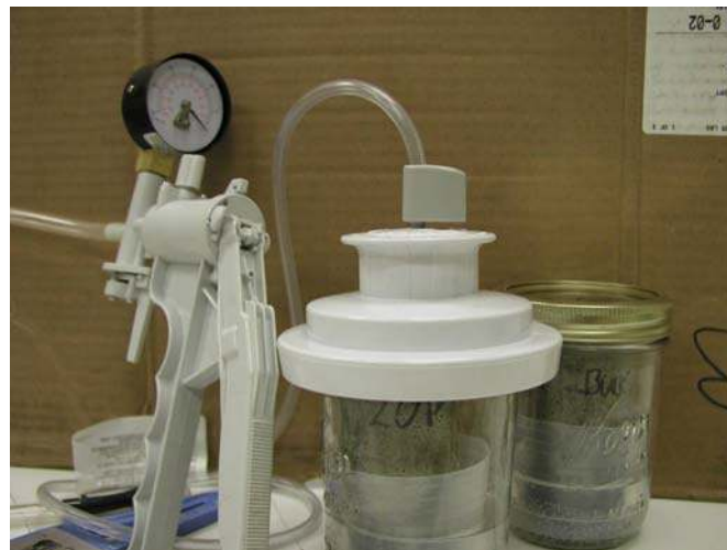
Figure 4-13 Vacuum Sealing of ASR cylinders for pore solution extrusion
