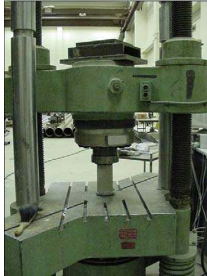
Figure 4-3 Cylindrical compression strength
