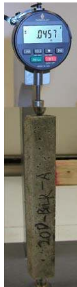
Figure 4-10 ASR bar length measurement (precision \pm 10^{-4} in)
