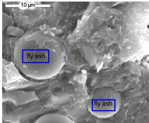
Figure 5-13 Barely reactive fly ash particle in Class F mix (56-day)
