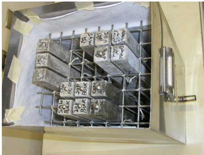
Figure 4-11 ASR bars cured in ASTM containers
