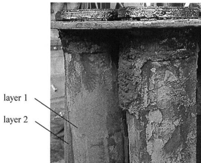
Figure 4-30. Ash deposition on the outside of the filter bags. Picture taken after two continuous runs without cleaning the filter unit. Two distinct layers can be identified.
