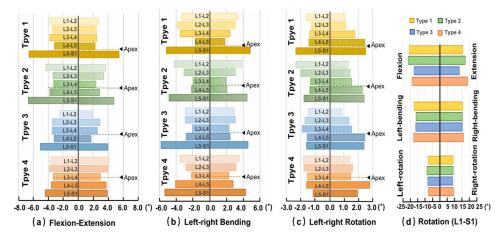
Fig 6. Rotation (°) of each segment of four Roussouly type FE models (a) in flexion-extension (7Nm), (b) lateral bending (7Nm), (c) axial rotation (5Nm) and (d) the L1-S2 segments in the six loading conditions.
