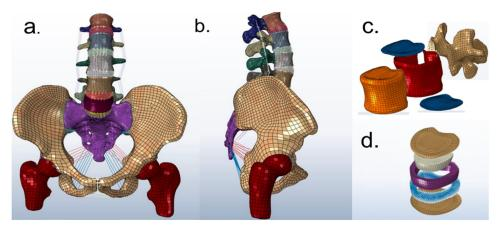
Fig 3. (a) Front and (b) lateral views of the FE model of the lumbar-pelvis; (b) Schematic of (c) the annulus fibrosis and (d) vertebra components.
