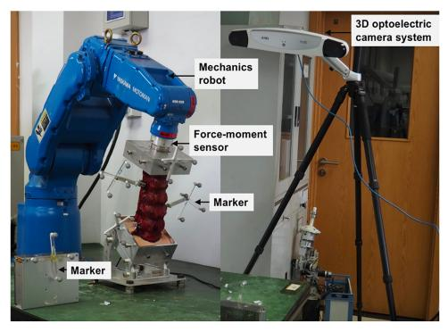
Fig 2. Image of the robotic testing device with a specimen embedded.
