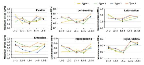
Fig 8. Maximum Von Mises stress of the annulus fibrous matrix of the lumbar-sacral segments in the four sagittal type models under all six loading conditions.
