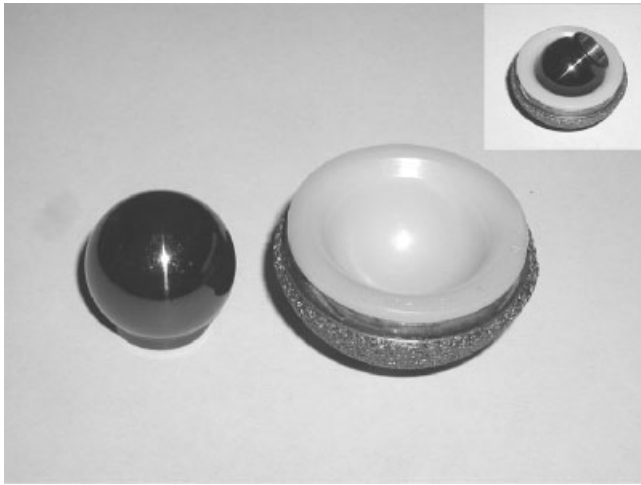
Figure 1. a-C:H coated head and UHMWPE acetabular surface of a hip joint by radio frequency plasma-assisted chemical vapor deposition.
