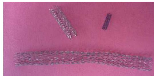
FIGURE 16: Example of SMA stents: (top right) coronary stent, (top left) carotid stent, (bottom left) femoral stent.
