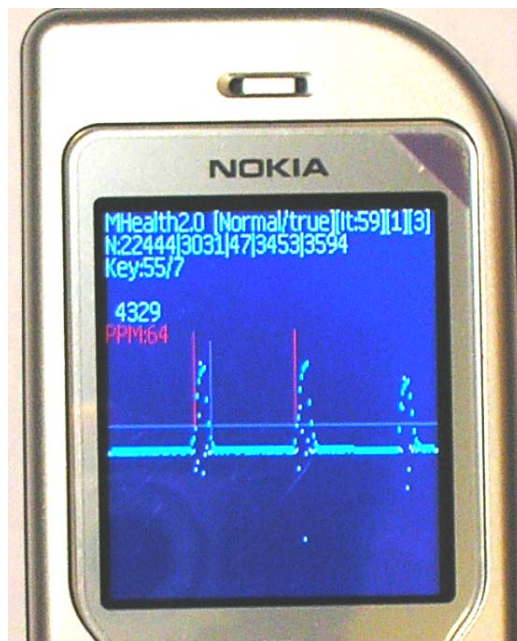
Figure 3. The graphical interface in the capturing state executing on a Nokia 6670 smartphone.
