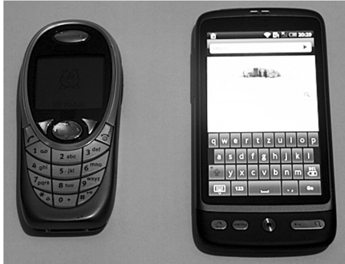
Figure 1. Left: hardware keyboard with a 12-key layout; right: software keyboard with a QWERTZ-layout
