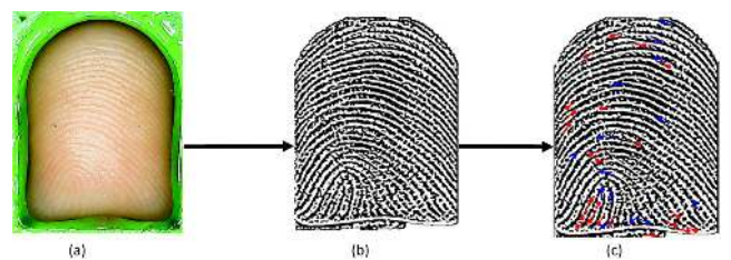
FIGURE 13. An illustration of the process from (a) the acquisition of the image of an infant's fingerprint, to (b) image processing to convert the fingerprint into a format which is compatible with commercial off-the-shelf comparison software, to (c) the extraction of minutiae points from the fingerprint.
