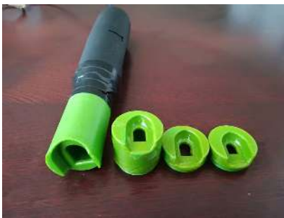
FIGURE 11. The contactless infant fingerprint acquisition device with different sized attachments to cater for varying sizes of children's fingers.
